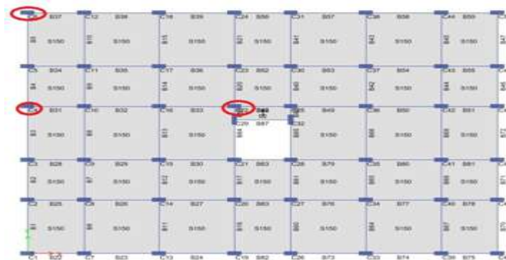
Fig. 1: Structural plan with (A4) and without (B4) staircase at centre location.
